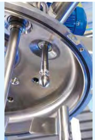
Spray nozzles for residue-free CIP cleaning
