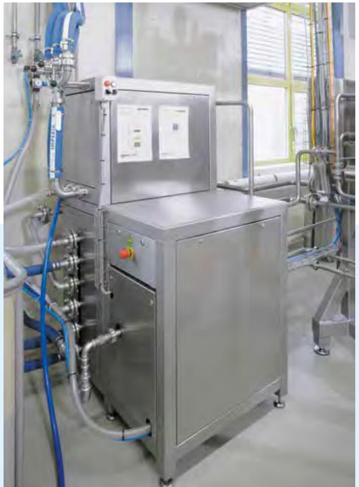
Separate supply unit with pneumatic and vacuum unit and liquid meters
