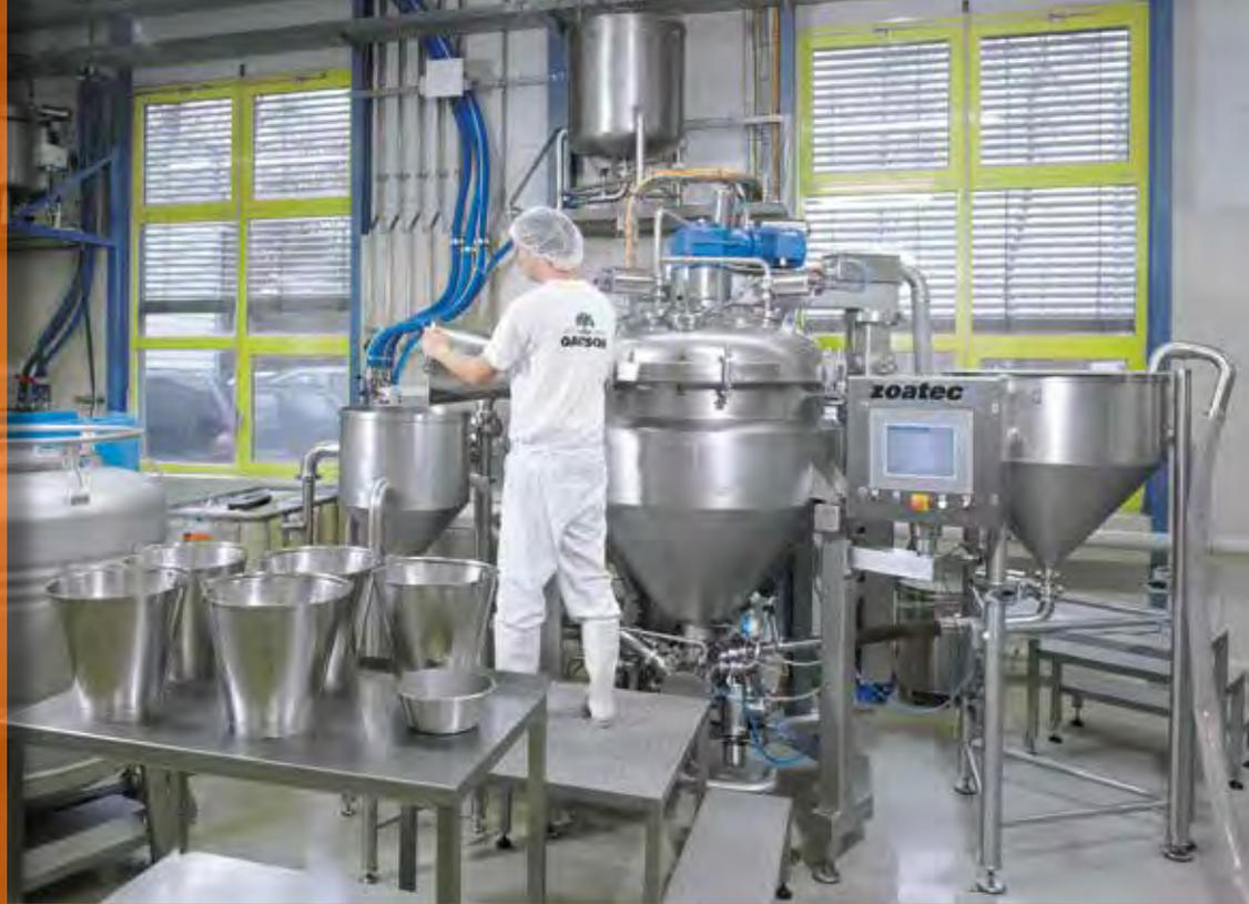
Feeding of powders and liquid premix via a feeding vessel
