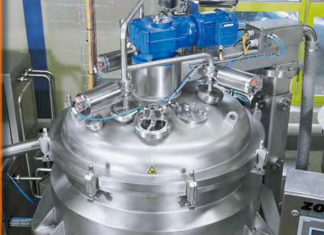
Lid with electrical lifting device
